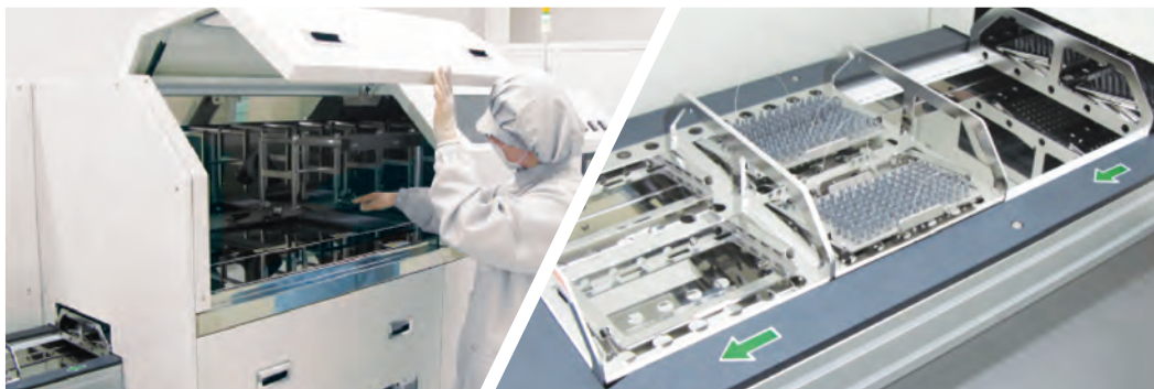
The cleansing process by ultrasonic wave using the 3rd distilled water, vacuum dry, and heating dry sterilization leaves no residue and ultimately sterilizes the products.
